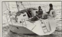
Hull length 28ft 6in 8.69m 7·14m 23ft 5in LWL 3.00m 9ft 10in Beam 3ft 9in 1.14m Draught 2,495kg 5.500lb Displacement Ballast 1,738lb 788kg Sail area 463ft<sup>2</sup> 43·01m<sup>2</sup> Engine Volvo 2001 6.7kW 9hp Berths
