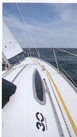
Inboard rigging allows a sensible sheeting angle for good pointing ability; the tacking angle is between 75 and 80°
