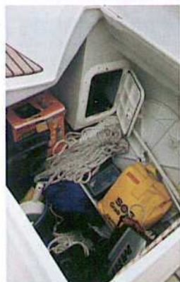
A separate gas locker is built into the main locker to starboard
