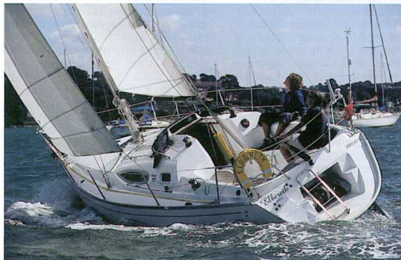
A recess in the transom provides stowage for the liferaft or inflatable dinghy
